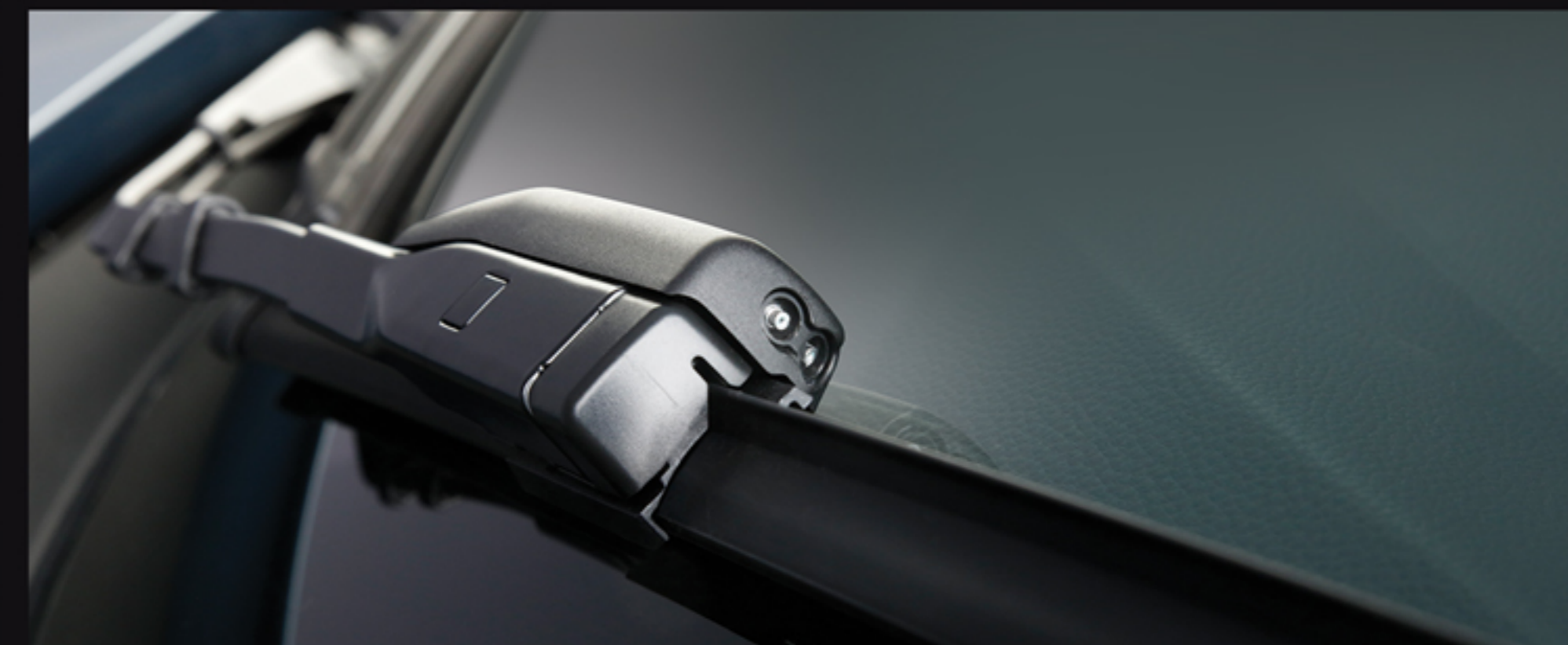
SMART CLEAR AUTO WIPERS: Water goes through the nozzles installed in the wiper for precise and detailed cleaning of the windscreen.
