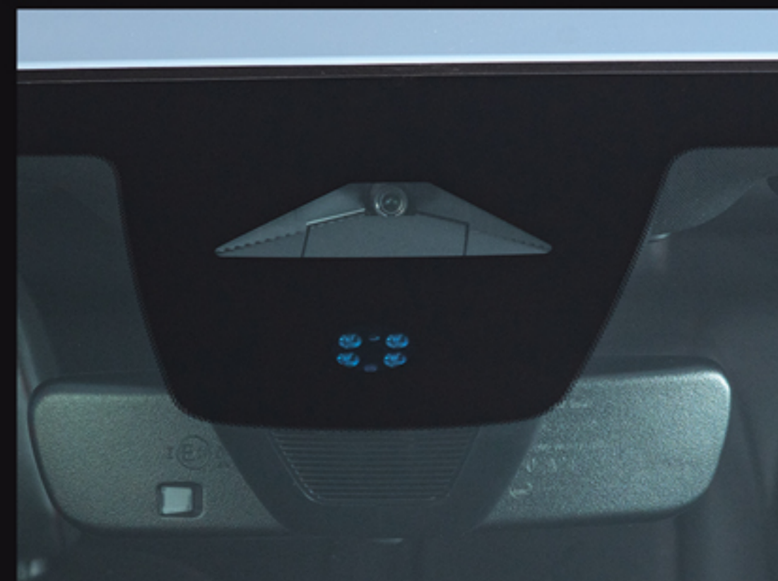
RAIN SENSOR: Automatically activate wipers.
