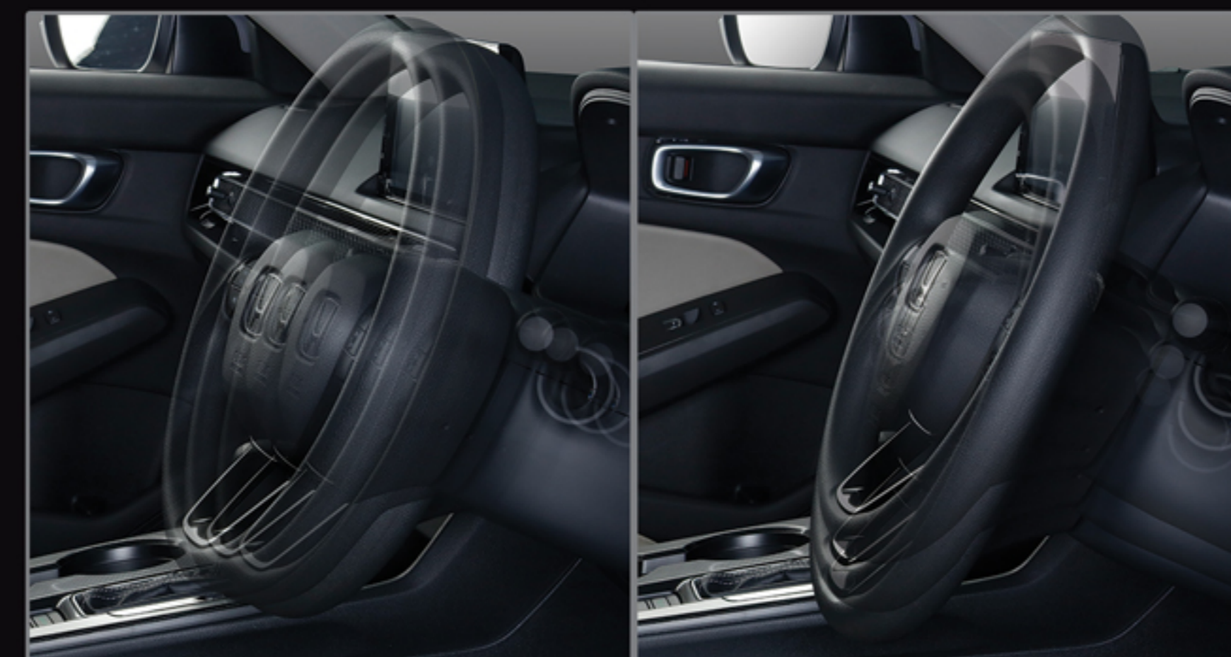
TILT & TELESCOPIC STEERING: Helps to adjust the steering wheel according to the driver's height by moving the wheel through tilted and telescopic movement.
