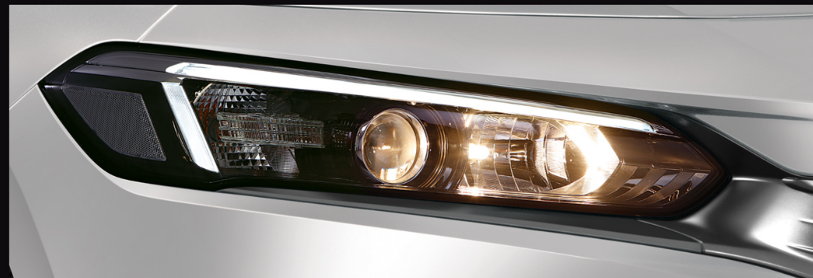
PROJECTOR TYPE HALOGEN HEADLIGHTS WITH LED DRL
