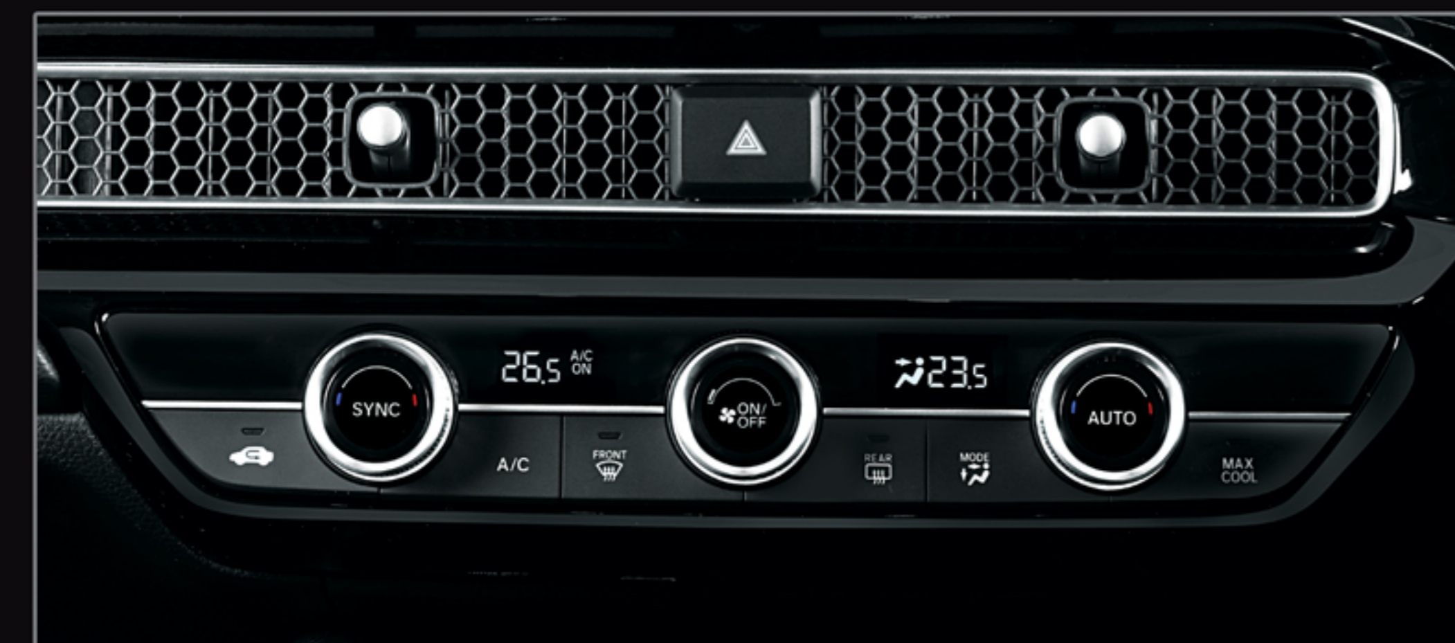
DUAL AUTO AC: Auto temperature control will ensure a pleasureable cabin throughout your trip with Drive/Assistance separate temperature setting.
