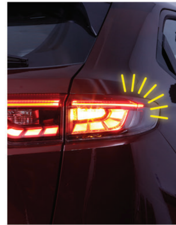
Emergency Stop Light
